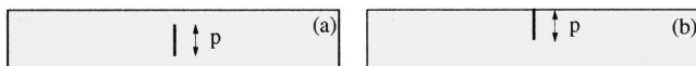
FIG. 4. Vertical crack in the aluminum plate; (a) internal crack symmetrical with respect to the middle plane of the plate, (b) opening crack.
