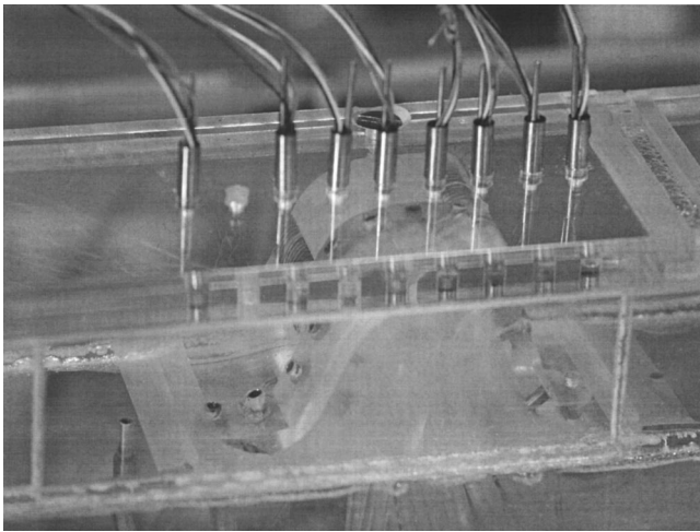
FIG. 3. Photograph of the glottis with positions of pressure taps on the vocal fold and eight pressure transducers within the flat upper wall.
